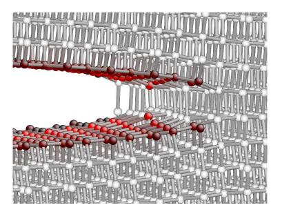
Slow crack propagation proceeds in three dimensions on the (110) cleavage plane in silicon through the formation and advance of kink pairs.
